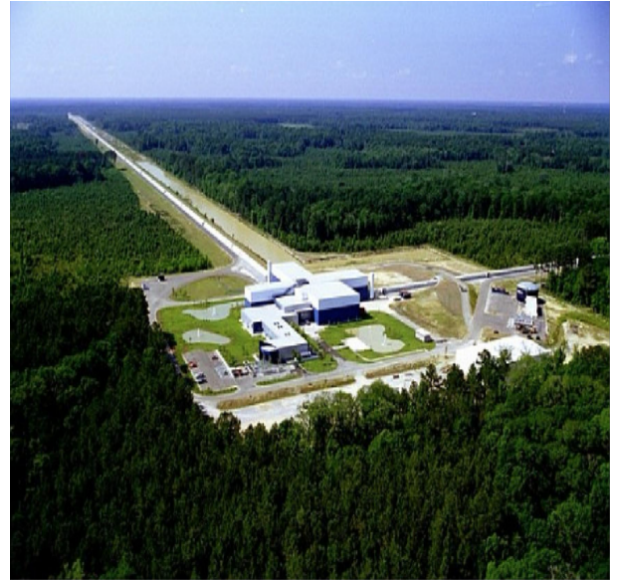
Figure 4: The Large Interferometric Gravitational-wave Observatory (LIGO) is, in essence, a Michelson interferometer; shown schematically at left. Photo at right is the detector at Livingston. The mirrors are suspended on fibres and so behave effectively like inertial test-masses. The Michelson interferometer is very sensitive to tiny changes in the lengths of the arms. If they are identical, no light comes out of the ‘dark-port’ as there is complete destructive interference. If they are changed slightly by the passage of a GW – which, for the appropriate polarisation – will stretch one arm and contract the other, some light will come out. The extra mirrors in the paths are to increase the effective distance the light travels in order to increase the sensitivity. With this set-up, the LIGO team are able to measure a strain of h \sim 10^{-21} . This corresponds to about 10^{-8} of the size of an atom!
